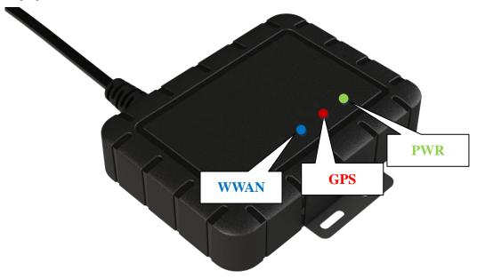
The following figure shows the location of AL11's LEDs.
